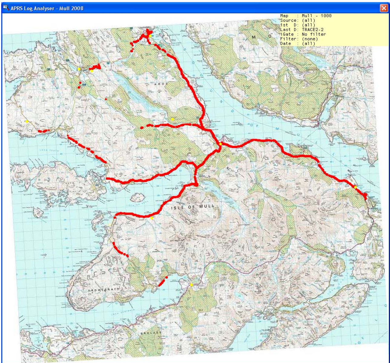
Radio coverage from Control
